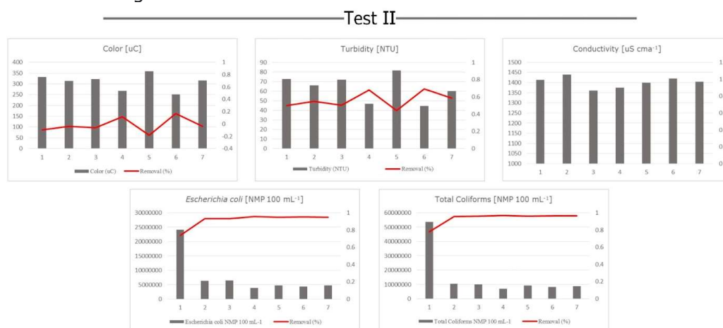
Fig.4. Removal efficiency of test II.
