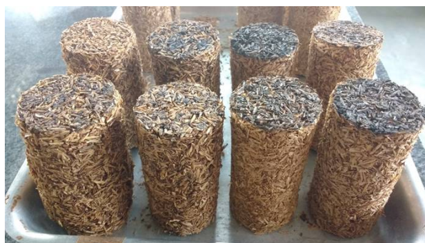
Fig. 1. Solid fuels made from rice husk biomass (30 g), mandarin peel (30 g), cornstarch (15 g), glycerol (10 ml) and acetic acid (5 ml).
