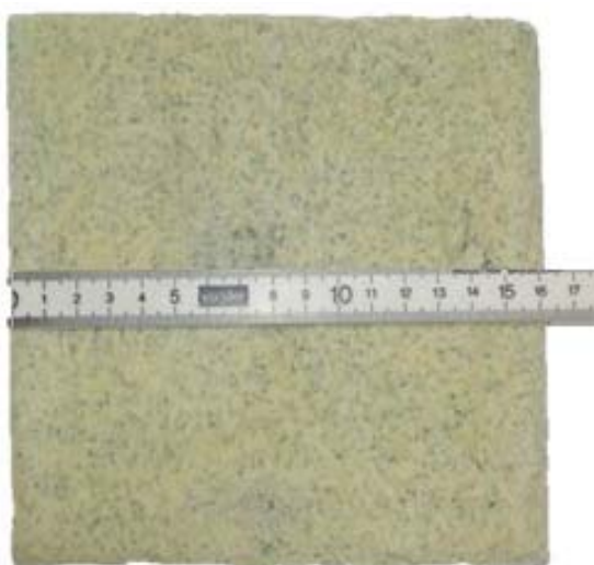
Fig. 1. Board composed of 5g polyol, 7.5 TDI, 12.5 g PET, 5 g AAS, and PU_AAS_50PET sample.
