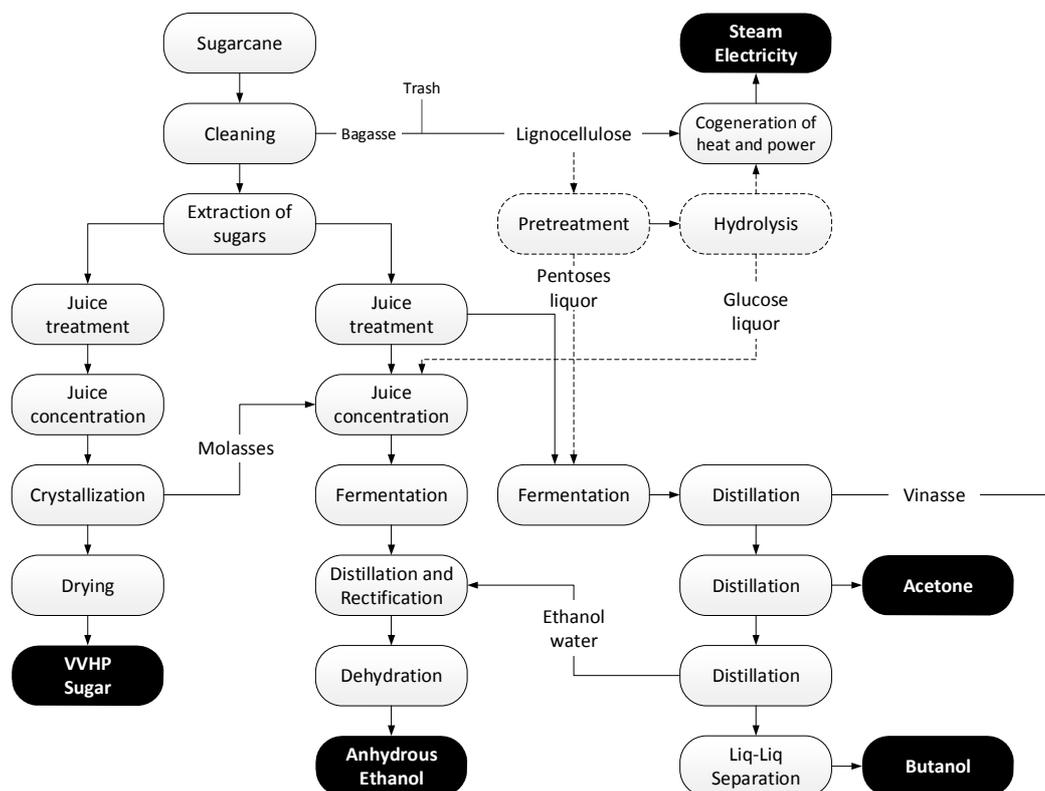
**Fig. 1.** Block flow diagram of integrated first and second generation production.
