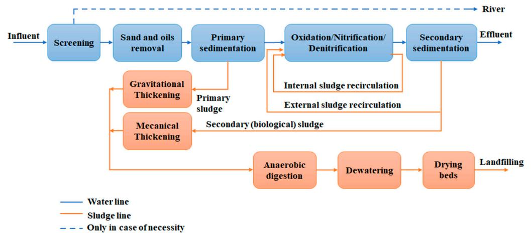
Figure 2. The Iași MWWTP flow-sheet (source: APAVITAL).
