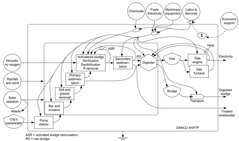
Figure 3. The Iași MWWTP’s energy-flow diagram. The \$ sign stands for the economic support needed for labor and services.
