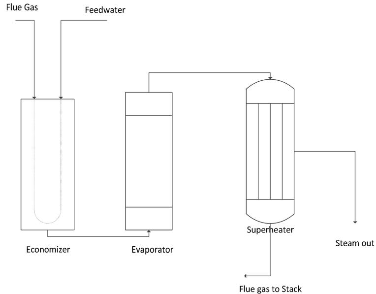
Fig. 3 - Steam production from incineration flue gas
