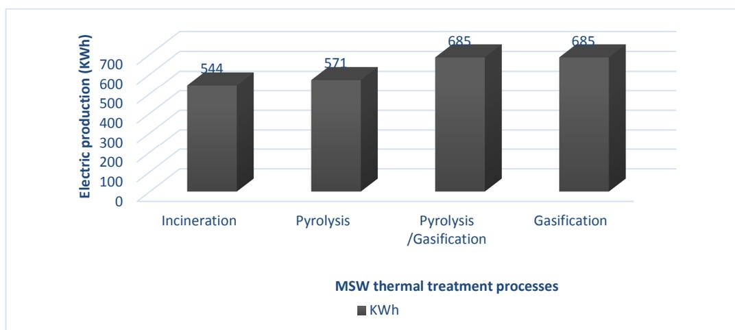
Fig.4- Thermal treatment processes energy generation per ton of MSW (C.Young, 2010)
