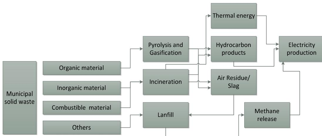
Fig.2 - MSW feestock separation and processing routes (A.U.Zaman, 2010)
