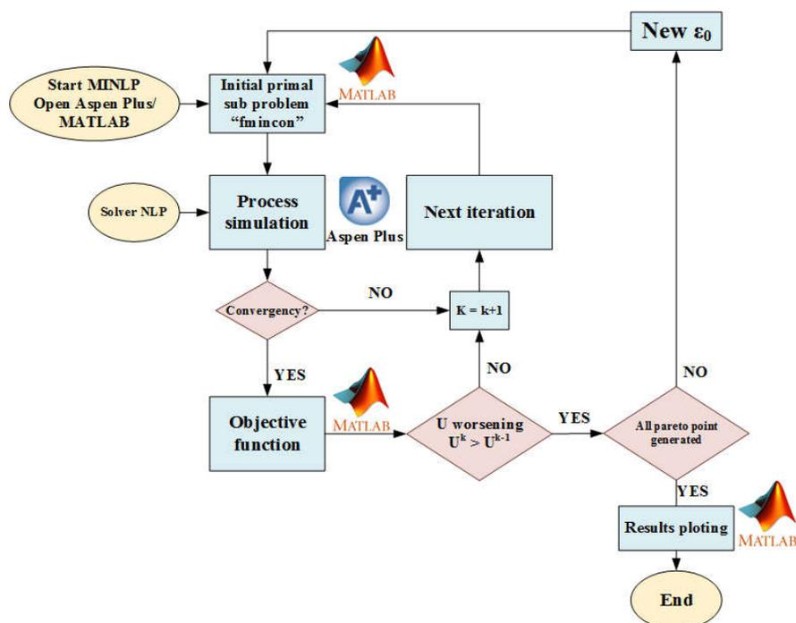
**Fig. 3.** Algorithm of the proposed methodology.
