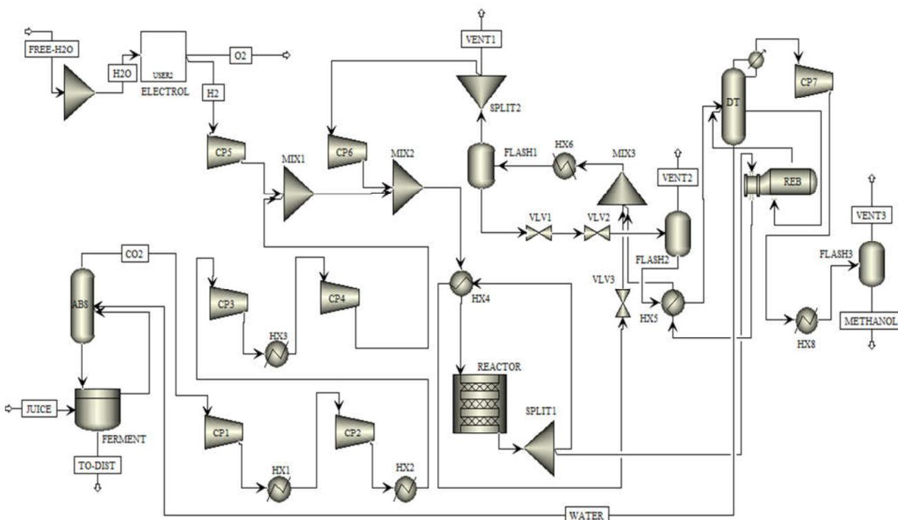
**Fig. 2.** Process flowsheet of the case study modelled in Aspen Plus v8.8.
