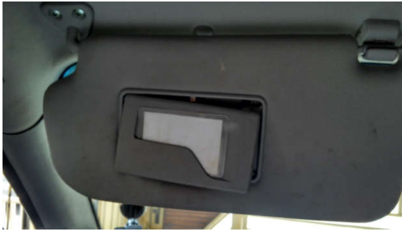
Fig. 2. Broken plastic support of vanity mirror in the sun visor of Hyundai Tucson, budgeted at almost 2% of the total car sales price to be replaced.
