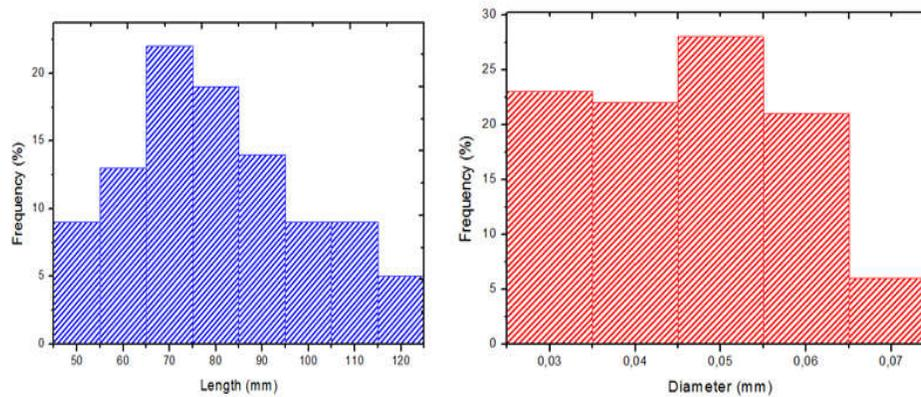
**Fig. 4.** Statistical distribution of the length and diameter of the hemp fibers
