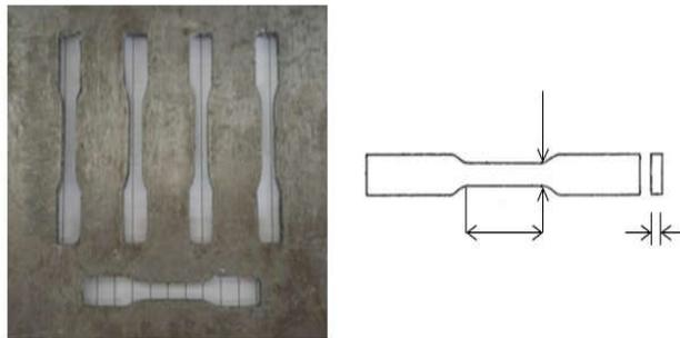
**Fig.2.** Metal matrix for tensile test
