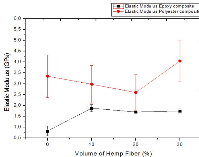
**Fig. 7.** Elastic Modulus of the epoxy and polyester composites in function different amounts of hemp fiber
