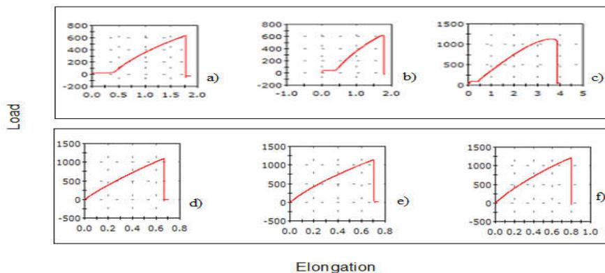
**Fig. 5.** Load curves vs. Elongation, obtained in the tensile test of the polyester matrix a) 0% reinforced with hemp fibers at b) 10% and e) 30% and of epoxy matrix d) 0% reinforced with hemp fibers at e) 10% and f) 30%.
