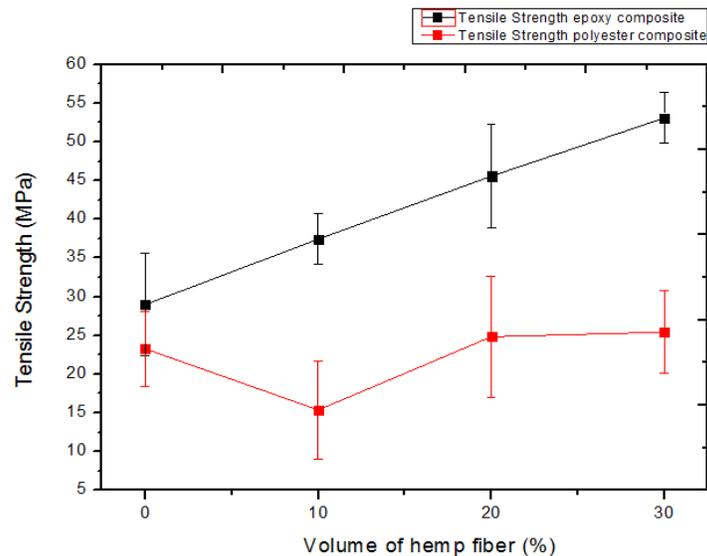
**Fig. 6.** Tensile strength variation with the amount of hemp fiber in the epoxy and polyester composites
