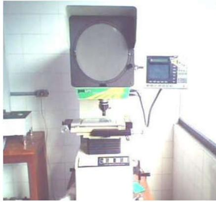
**Fig.3.** Nikon Profile Projector used to measure fiber diameters
