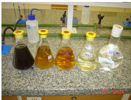
Fig. 7 – Leachate cleared with coagulation-sedimentation process with a stage of filtration with active carbon
