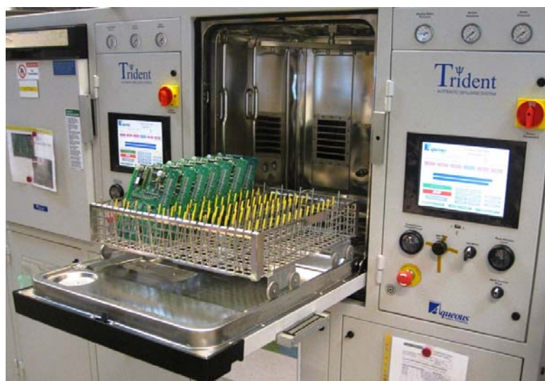
Fig. 3. The first installed application and usage of the Qlean-method within the electronic industry – cleaning of printed circuit boards.
