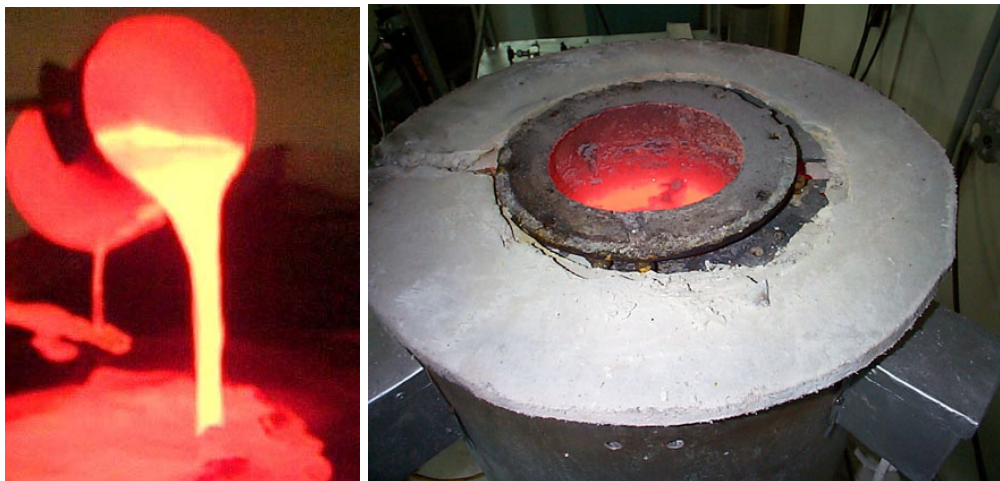
Figure 3: molten salt (left) and the reactor opened (right) containing the molten salt.
