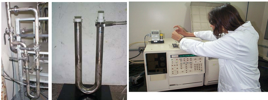
Figure 5: Gas sampling system (left and center) and CG/MS analysis (right).
